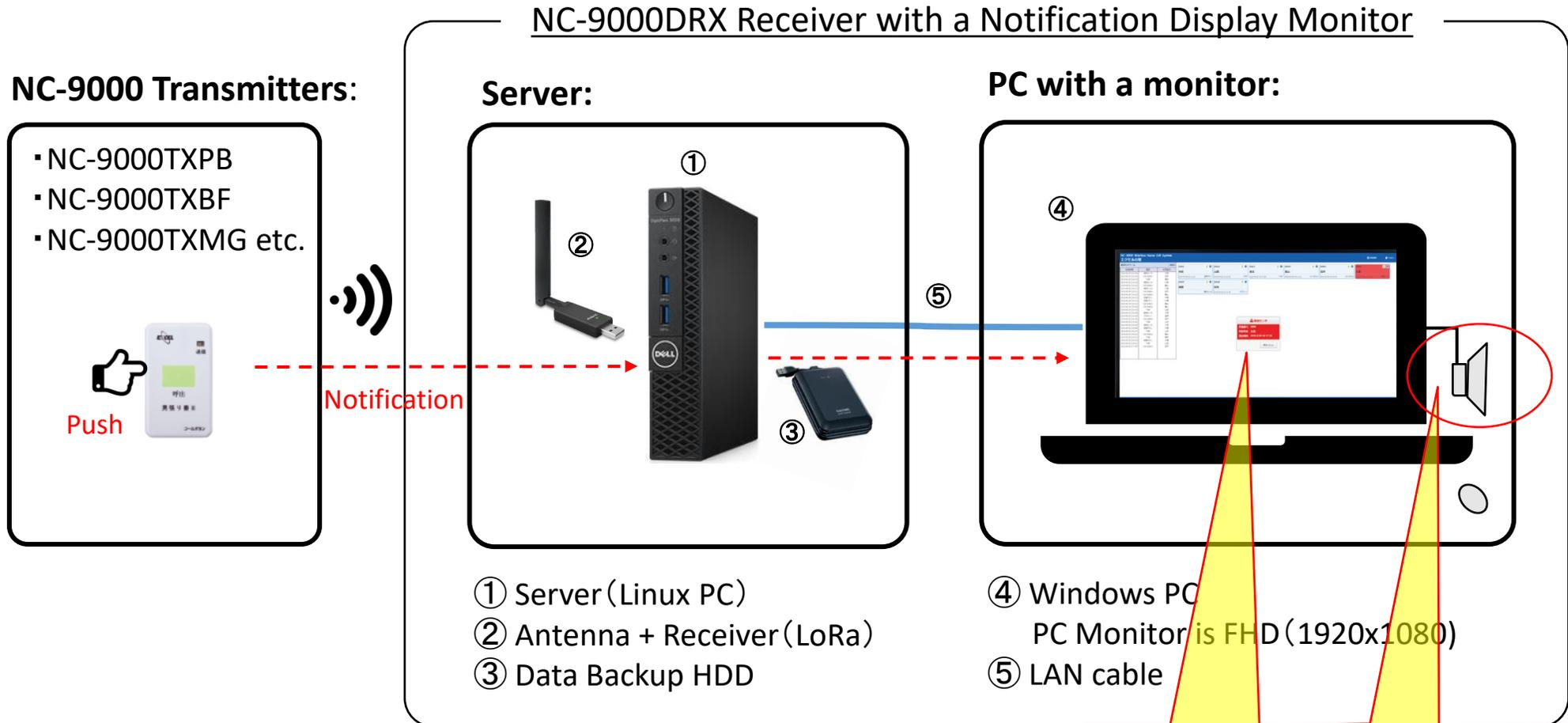
\*The red lines represent how the alert signals are routed.
